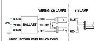
The wiring diagram that appears above is for the lamp type denoted by the asterisk  $(\ensuremath{^*})$
