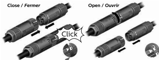
Automatic locking mechanism
