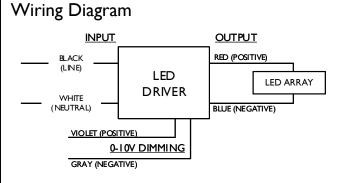
Input, Output and 0-10V Dimming use lead-wires. Input & Output Lead-wires are 18AWG 105C/600V solid copper. 0-10V Dimming Lead-wire is 22 AWG 105C/600V solid copper.
