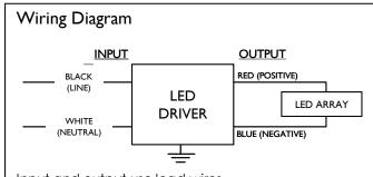
Input and output use lead-wires. Lead-wires are 18AWG 105C/600V solid copper
