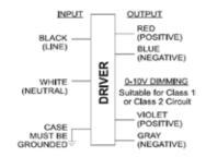
Input and output use lead-wires.
