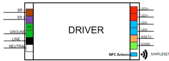
Figure 3. Driver connector color code definition
