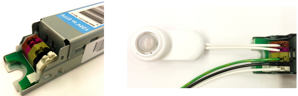
Figure 8. Driver input-side showing SR connector (left) and two-wire connection to a radio sensor (right)
