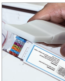
LED driver with SimpleSet technology
