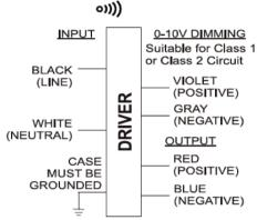
Input and output use lead- wires.
