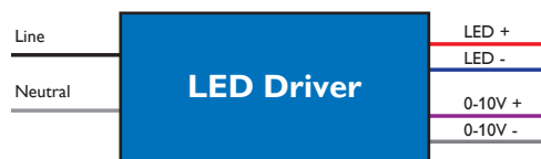
Figure 7. LED driver with 0-10V dimming interface.
