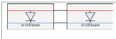
Schematic representation of the wiring of 2 connected LV LED boards, not needing a Return-End cable
