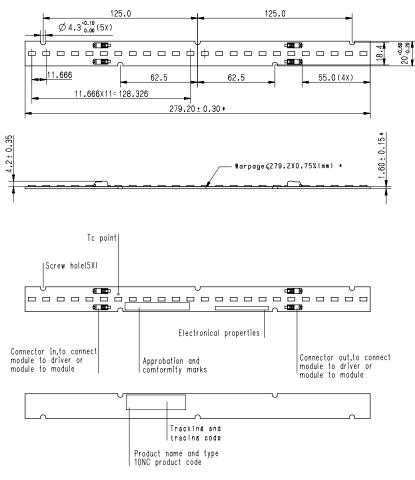
Un-indicated tolerance see ISO-2768-m Not specified inner R Angle unity is 0.5mm
