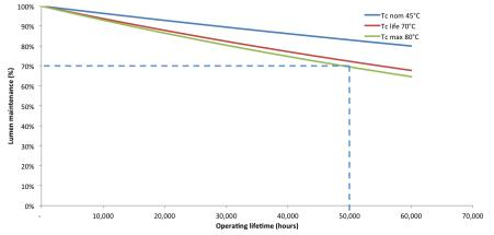
Lumen depreciation as a function of operating hours at different Tc values and I-life. 36,000 hours proven by certified laboratory.
