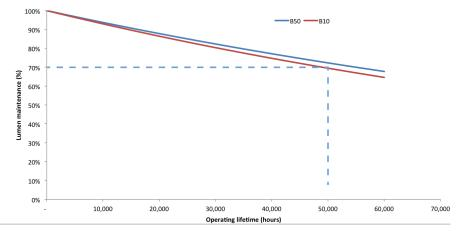
Lumen depreciation as a function of operating hours for I-life and Tc-life. 36,000 hours proven by certified laboratory.
