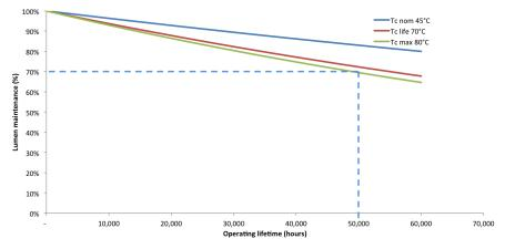
Lumen depreciation as a function of operating hours at different Tc values and I-life. 36,000 hours proven by certified laboratory.
