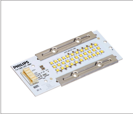
Figure 2. Fortimo LED HBMt Gen3 6000 lumen
