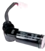
PC3 Plug-in photo cell, 3" (78mm) lead for direct mount to transformer housing.
