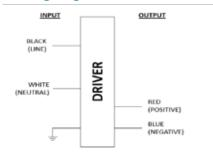
Input and output use lead- wires.
