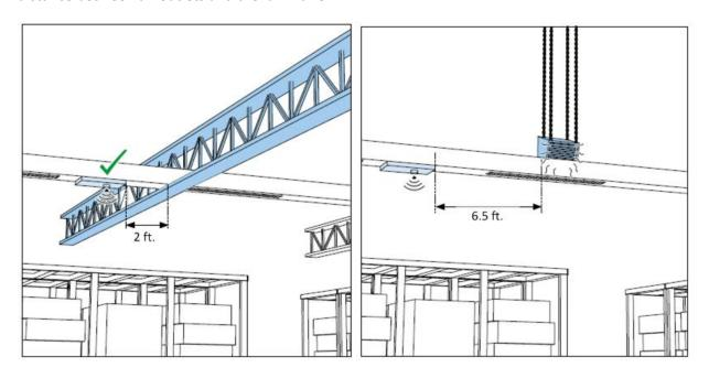
Also check that the first luminaire is in the right position and oriented correctly with respect to the edge of the isle. Refer to section 12 (walk test) for details on testing the coverage area of the sensor. Note the luminaire needs to be grouped before performing the walk test.
