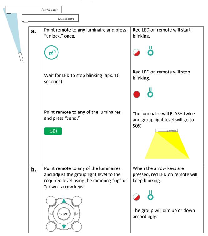
Press the "save" button, the light level is Red LED on remote will blink. C. stored as a new daylight set-point. The entire group will FLASH twice and group light level will go to 50%. Luminaire Point to any of the luminaires in the Red LED on remote will start d. group and press "lock." blinking. The luminaire will FLASH twice. Wait for LED to stop blinking (apx. 10 Group is ready for normal seconds) then press "send." operation. Luminaire 0)))
