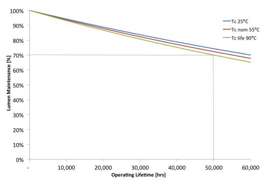
Lumen depreciation as a function of operating hours for I-life and Tc-life. 50,000 hours proven by certified laboratory.
