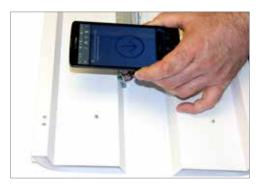
Step 1: Place the smartphone next to the NFC antenna on the driver.
