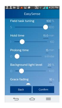
EasySense parameters can be configured via Philips field apps. You must first register for the app to receive a username and password, then download Philips field apps from the Google Play Store. Refer to www.philips.com/easysense for details including applicable Android phones.
