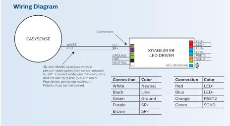
Note: Refer to www.philips.com/easysense for quick installation guide.
