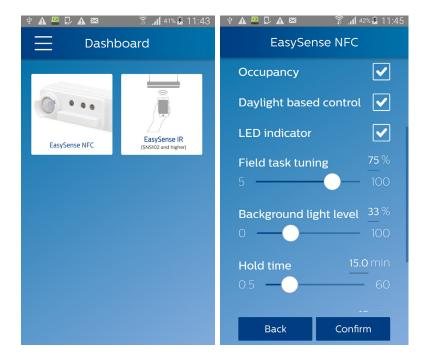
EasySense parameters can be configured via Philips field apps. Two versions are available:
