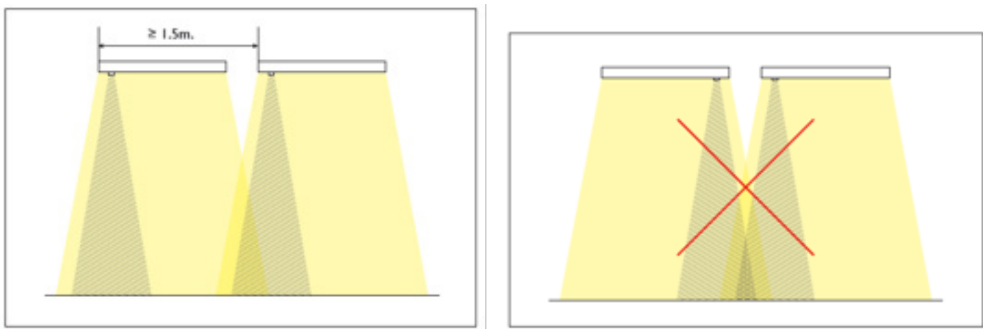
Figure 14. Distance between sensors should be at least 1.5m apart.
