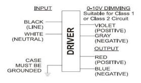
Input and output use lead- wires.
