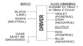
Input and output use lead- wires.
