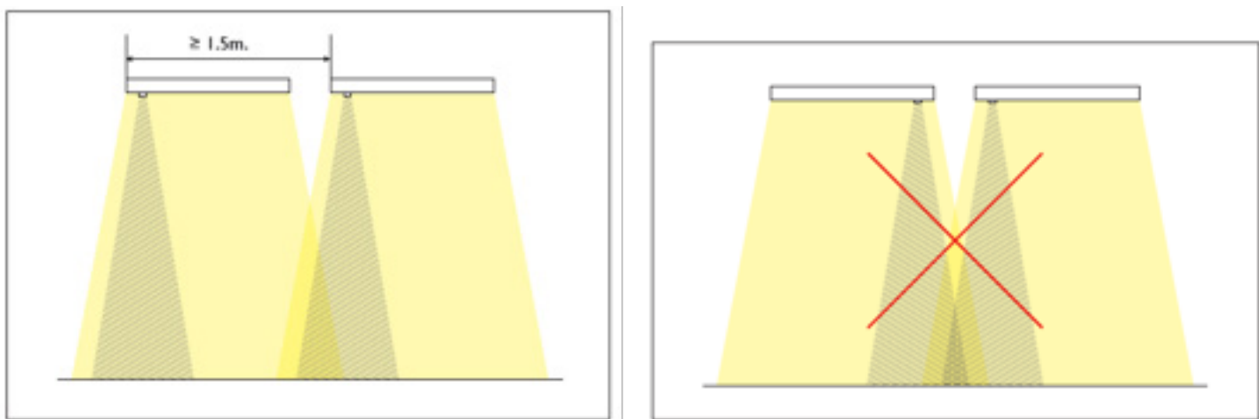
Figure 25. Distance between sensors should be at least 1.5m apart.
