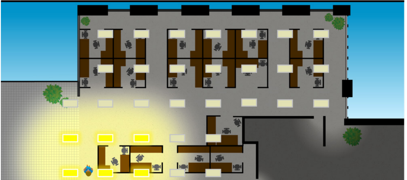
Figure 13. Light adjusts as room occupancy changes.
