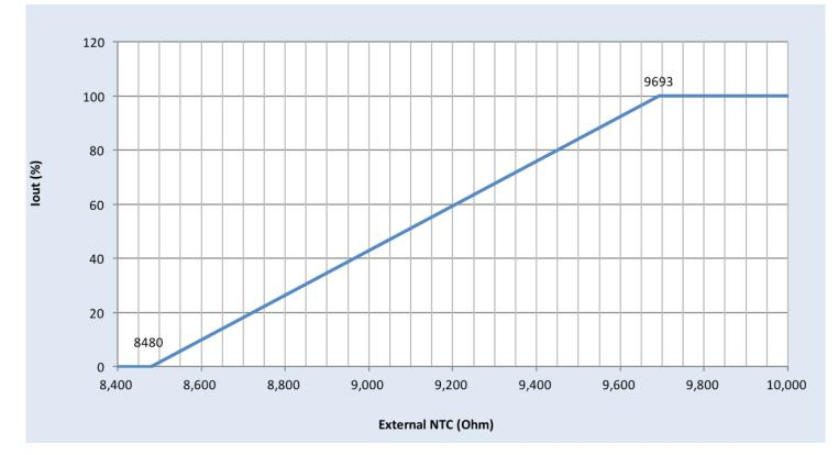
Output Current Vs. LED Module Temperature Using 100kohm NTC
