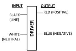
Input and output use lead wires.
