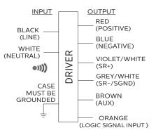
Input and output use lead-wires.
