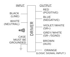
Input and output use lead-wires.
