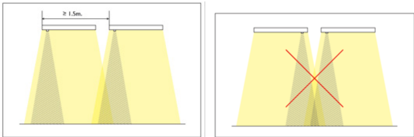
Figure 13. Distance between sensors should be at least 1.5m apart.
