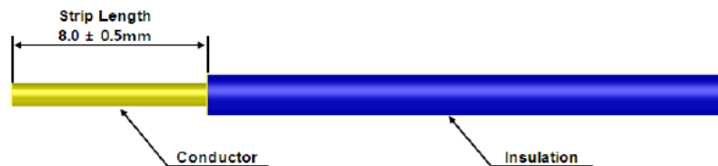
Figure 7: Wire strip length.
