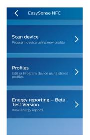
Place the back of the smartphone (where the NFC reader is located) onto the sensor NFC antenna (almost touching) to enable NFC communication. NFC communication might take a few seconds. Do not move until you hear a beep and the next screen appears.
