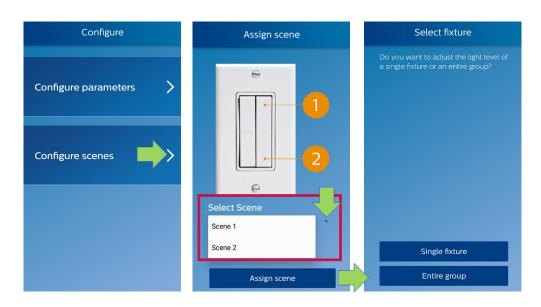
The scenes are selectable via the scene buttons of the switches associated either to fixture or an entire group.
