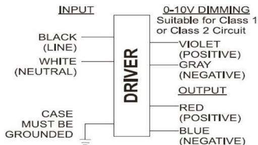
Input and output use lead- wires.
