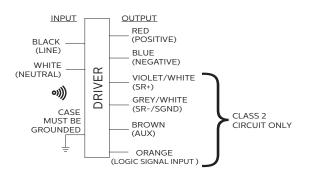
Input and output use lead-wires.
