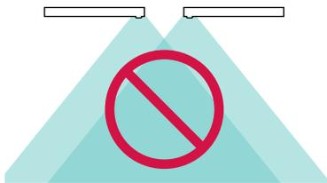
Ensure sensors from adjacent luminaires are not positioned next to one another.
