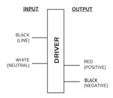
Input and output use lead wires.
