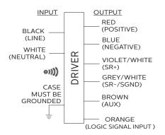
Input and output use lead-wires.
