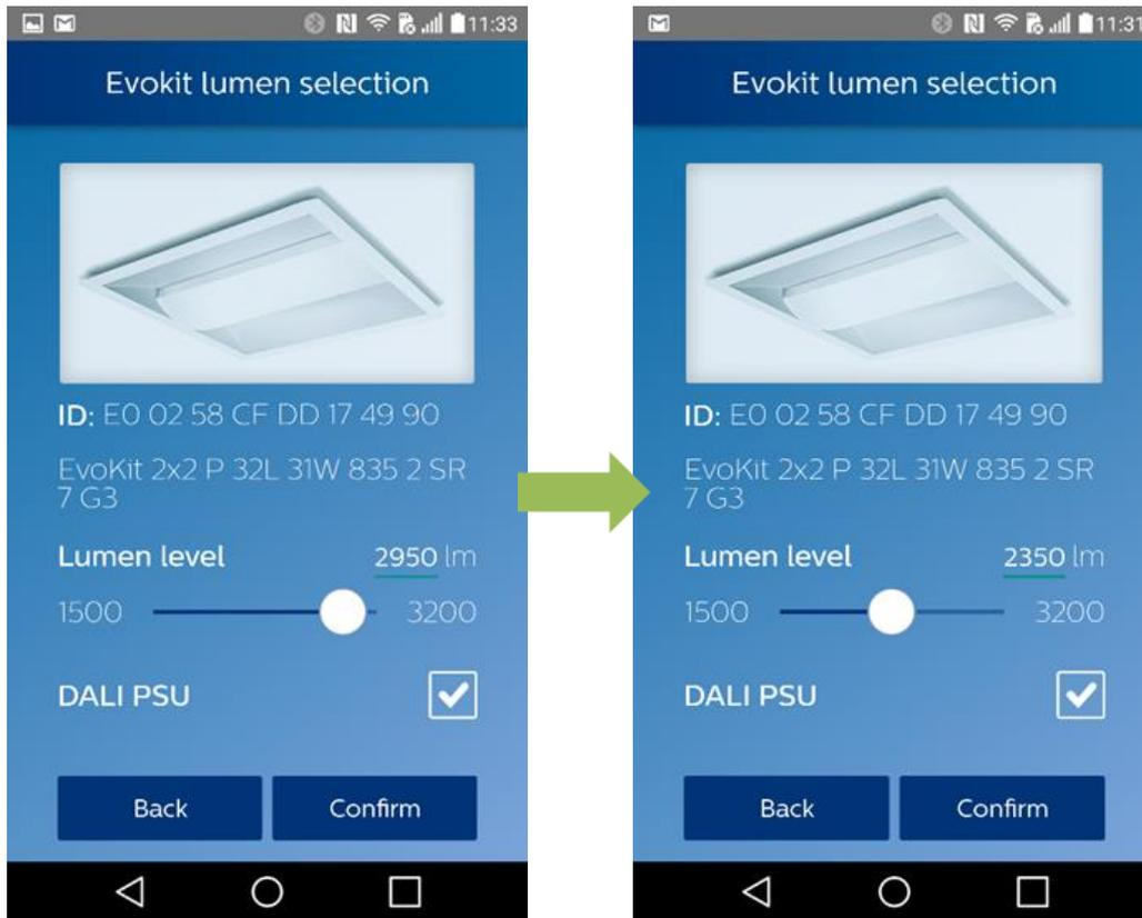
NOTE: The 'DALI PSU' checkbox will only appear for EvoKit SR units. This box should always be checked when using a sensor.
