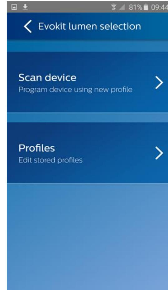
3. Touch the back of the smartphone onto the SR driver NFC blue antenna to enable NFC communication. NFC communication might take a few seconds, do not move until next screen shows.
