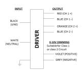
Input and output use lead- wires.
