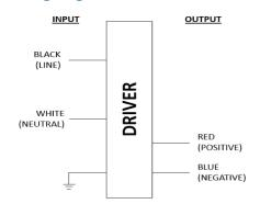
Input and output use lead- wires.
