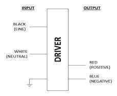
Input and output use lead- wires.
