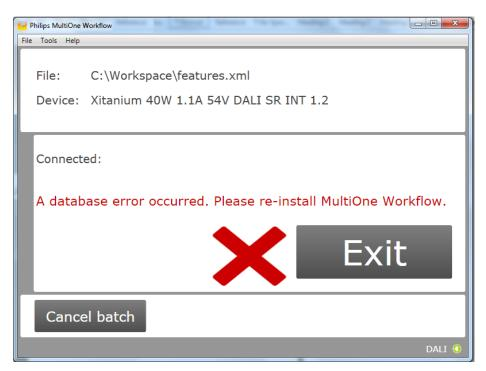
Click **Exit** to close the application window and re-install the MultiOne Workflow.
