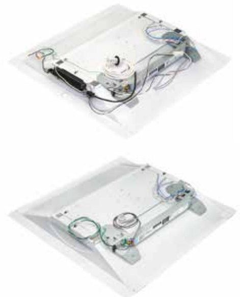
Separate components add unnecessary complexity to luminaires (top), while Xitanium SR LED drivers integrate many of the components (bottom) for a streamlined luminaire design.
