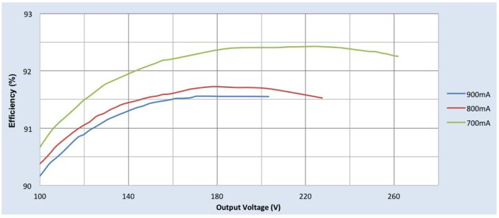
Efficiency Vs. Output Voltage at 277Vac
