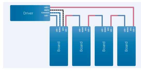
If a system consists of multiple Fortimo FastFlex boards connected to a single driver:
