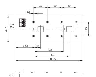
FastFlex LED module assembly
