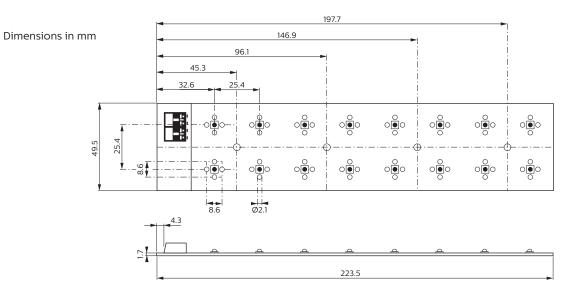
FastFlex LED module assembly
