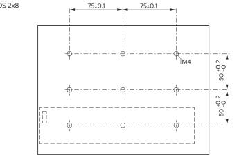
Mounting hole pattern for FastFlex DS 2x8
