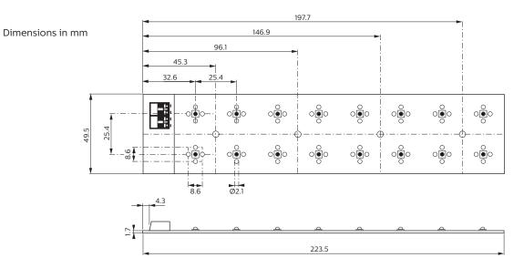
FastFlex LED module assembly Mounting hole pattern for FastFlex DS 2x8
