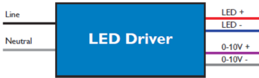
Figure 6. LED driver with 0–10V dimming interface
