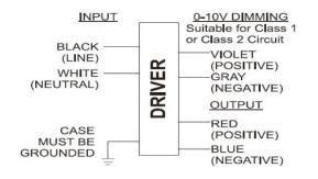
Input and output use lead- wires.
