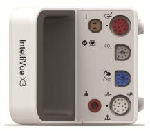
The  $SpO_2$  option shown above is the Philips FAST  $SpO_2$ . It is the only  $SpO_2$  option that can be combined with the built-in  $CO_2$  or a second Philips FAST  $SpO_2$ . Also available are:
