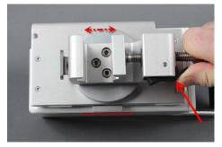
2 Turn the handle to screw the mount securely into place.
