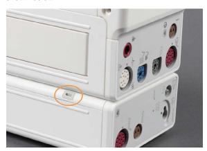
If this is the case, the plugs must be removed with a screwdriver before the measurement extension can be separated from the monitor.
