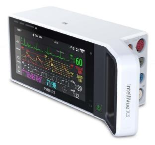
The IntelliVue X3 is a versatile patient monitoring device with a color touchscreen display. It can simultaneously monitor ECG (using 3-, 5-, 6- or 10-lead sets, including arrhythmia and ST monitoring), respiration, SpO<sub>2</sub>, NBP, two invasive pressures, temperature, and CO<sub>2</sub>. The multi-touch screen allows easy interaction by swiping and tapping with one or two fingers.
