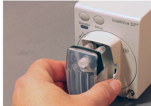
Installing the water trap
